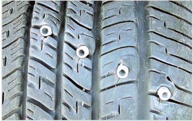
The barbs of a stop stick are shown in a tire that has been punctured.
